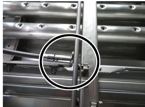
4. Loosen the cap nuts.
