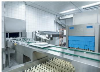
MEIKO bi-cord conveyors can even be used in locations where space is tight or the layout is challenging. This is the perfect type of conveyor system for situations that involve slight changes in height, for example:
