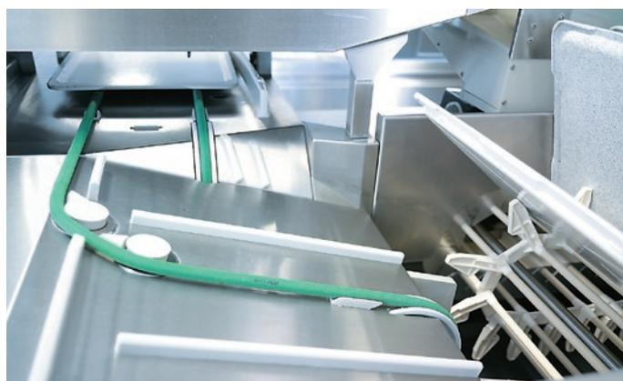
Key features of MEIKO's automatic dishwashing systems include automatic tray infeed and automatic cutlery transfer using a cutlery lifting magnet.
