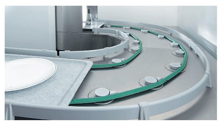
Round-belt conveyor technology can conquer any possible type of curve. Differentiated speeds and the necessary spacing carry the trays safely and securely around the curve in the centre of the conveyor. High, sturdy tray guides ensure that any dishes which are stacked tightly do not fall off at the corners, as well as safely and securely steering the trays.
