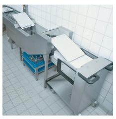
**Cutlery transfer without cutlery lifting magnet:** Trays are tipped so that cutlery falls into a cutlery basket. The empty trays are carried up a sloping conveyor to the tray stacking device.
