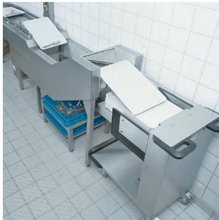
**Cutlery transfer without cutlery lifting magnet:** Trays are tipped so that cutlery falls into a cutlery basket. The empty trays are carried up a sloping conveyor to the tray stacking device.
