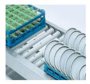
A roller conveyor automatically brings racks or containers to the machine at the correct rate.
