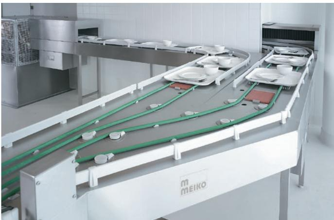
The MEIKO multifunction switch shown above provides additional functionality: at full capacity, two conveyors can run at 2 x 30 trays/min – but at low demand or during maintenance works, a mode can be activated which moves trays from both (incoming) conveyors to just the selected one of the conveyors for the next section – at a capacity of up to 30 trays/min. The capacity of the incoming sections can differ so long as the combined total does not exceed 30 trays/min.
