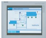
A central control cabinet is a key feature of every MEIKO conveyor system. Here, a schematic representation of the conveyor system's route with all components and modules give staff a clear overview of the system, even if it is long and complicated. For further visual options and analysis, the control station can also be fitted with a touchscreen. Intuitive operation facilitates excellent monitoring and control of the whole conveyor route. Different user levels, saved
