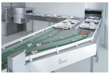
The MEIKO multifunction switch shown above provides additional functionality: at full capacity, two conveyors can run at  $2 \times 30$  trays/min – but at low demand or during maintenance works, a mode can be activated which moves trays from both (incoming) conveyors to just the selected one of the conveyors for the next section – at a capacity of up to 30 trays/min. The capacity of the incoming sections can differ so long as the combined total does not exceed 30 trays/min.
