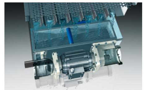
With food waste removed from the system, the wash water is cleaner and more effective – and no extra water is required.
