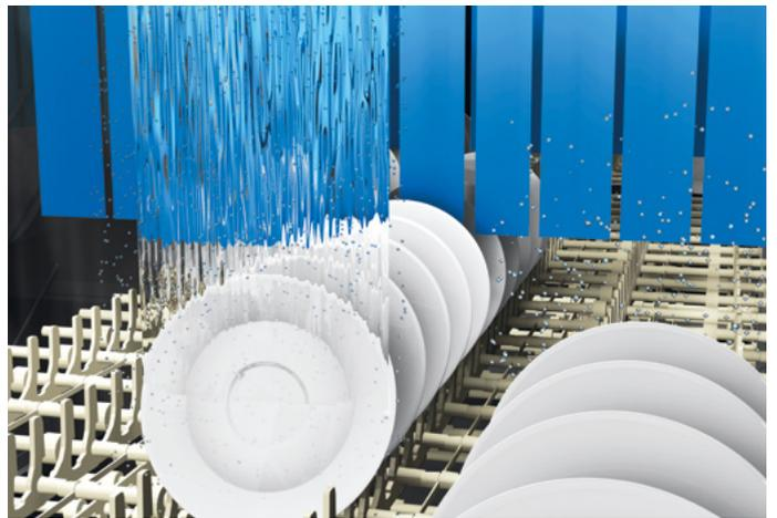
The final rinse function is only activated for sections of the belt that actually contain dishes.
