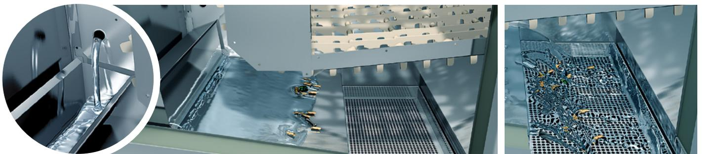
The machine collects the process water and then uses powerful torrents of this water to wash food waste into the scrap screen.
