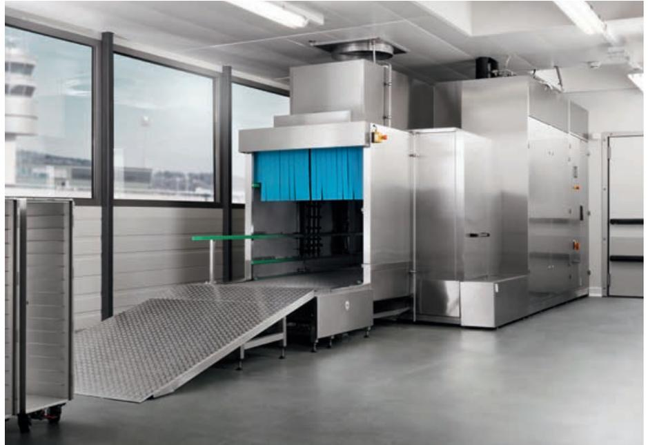
Easy loading – With a ramp height of only 400 mm, little effort is necessary to roll a full-size meal trolley onto the heavy-duty stainless steel belt, which transports the trolley through the washer, with little effort.
