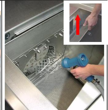
Lift the flap and use a water hose to flush out the tank and the shredding mechanism, if possible with warm water.
