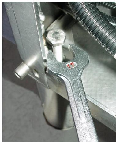
When the appliance is finally positioned, you must ensure that all the cleats carry approximately the same weight.
