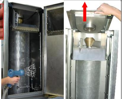
Open the tank cover and the cleaning door of the wet waste press. Flush out the interior of the press. Open the cover of the wet waste press.
