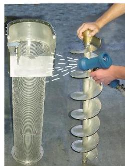
Remove the screen tube and the worm spindle and pull them apart. Both parts can now be cleaned easily, e.g. on the floor plate.
