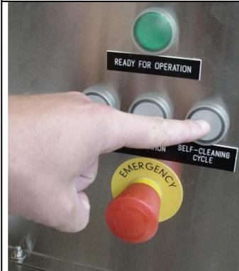
Press the "OFF" button for the final cleaning cycle. After approx. 15 min. this cycle is terminated automatically.
