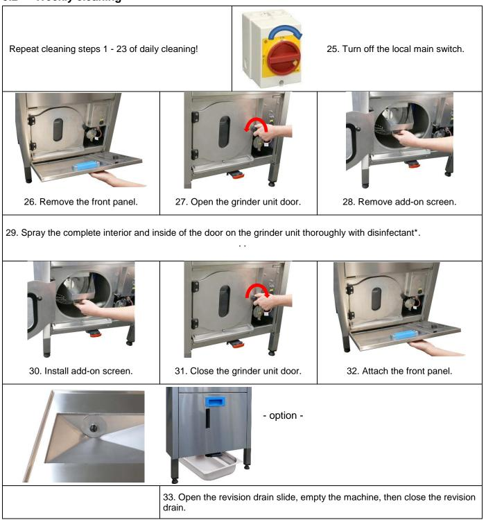
Any safety covers that must be removed in order to perform such operations must be returned to their original condition when the work has been completed.
