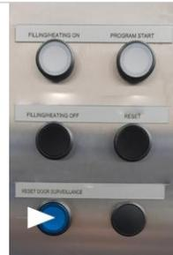
Press the **RESET DOOR SURVEILLANCE** button after having loaded the installation with wash ware and closed the doors.
