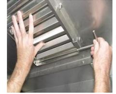
Remove the condensation separator.
