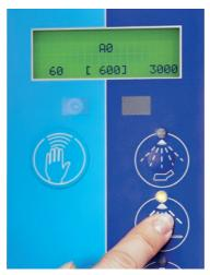
The display shows the available A<sub>0</sub> settings: A<sub>0</sub> 60 / A<sub>0</sub> 600 / A<sub>0</sub> 3000. Release the button when your setting appears.
