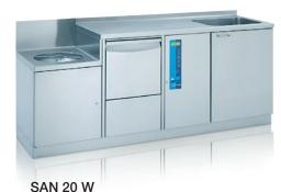
Combined care unit with 600 mm cupboard space. Consists of *TopLine 40*, slop sink, washbasin and storage surface. Includes splash screen and upstand.
