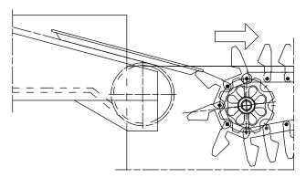
If the tray runs against the tray transport finger during infeed (see illustration below), the disc **must** be turned slightly **opposite to the transport direction**.
