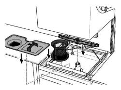
6. Insert filter, tank cover sieve and wash systems (top and bottom).
