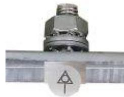
The screw for the equipotential bonding is located behind the cover on the front of the machine.
