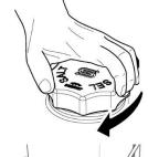
2. Clean the seal and thread of the salt solution container and close tightly. The ingress of wash water can cause capacity loss in the water softener!
