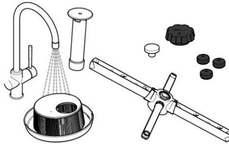
2. Remove filter, wash systems below and rinse arm above. All parts to be cleaned are blue or have a blue handle.
