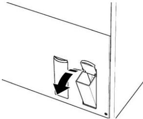
1. Swing the corresponding tank down for filling and open the cover.
