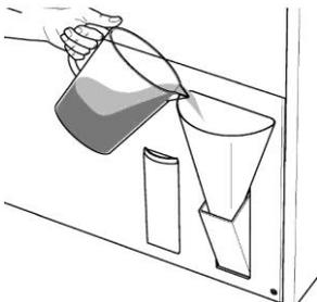
3. Use the loading chute to pour the chemical carefully into the tank until full. Check fill level.
