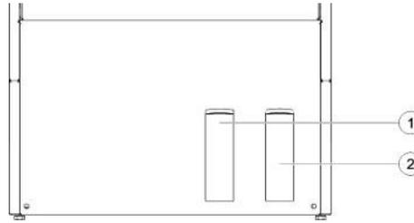
The storage tanks are located on the front of the lower front panel. The fill level can be read from the front. The detergent tank (1) is transparent, the rinse aid tank (2) is blue.
