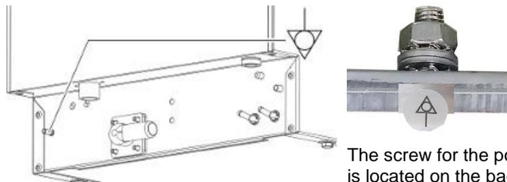
The screw for the potential equalisation is located on the back of the machine near the media connections.
