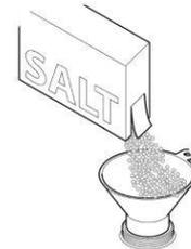
1. Open door, open salt solution container and fill with 1.5 kg of regeneration salt (sodium chloride with a grain size of 0.3 - 1 mm). If possible, use a loading chute!
