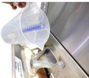
3. Use the loading chute to pour the chemical carefully into the machine until the storage container is full. Check fill level from outside.
