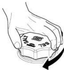
2. Clean the seal and thread of the salt solution container and close tightly. The ingress of wash water can cause capacity loss in the water softener!
