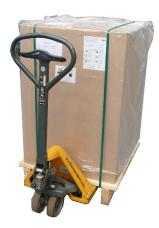
Only transport the device in its original packaging, otherwise it will not be stable during transport. Square timber frame (pallet) has additional cross struts at the bottom for stabilisation on lifting forks during transport. Only transport with lift truck!
