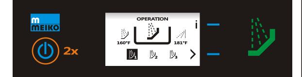
Press the 🕛 button TWICE to switch off the machine.
