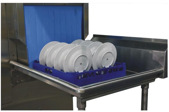
Load plates, soup bowls, etc. at an angle with the inside face pointing up. Ensure that water can drain correctly without pooling in hollow areas in the ware.
