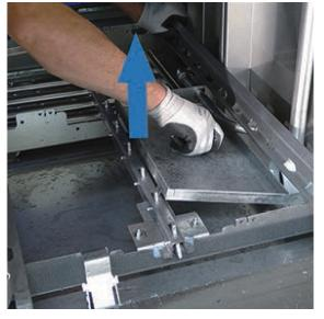
Remove the drain standpipe while touching the handle only to empty the tank(s).
