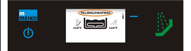
Wait for the machine to finish filling. 🦻 will flash as the machine fills, and the display will read FILLING/HEATING.
