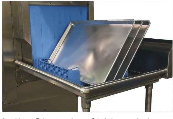
Load large, flat ware such as cafeteria trays or sheet pans facing front - so that the edges enter the machine first. Cafeteria trays may be loaded into a standard peg rack. Sheet pans **MUST** use an open-ended sheet pan rack as shown (with the back of the pan extending past the rack).
