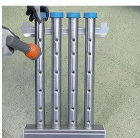
Thoroughly spray all scrap screens, rinse arms and splash curtains using a spray hose. Set all components aside in a clean, dry area to dry overnight.
