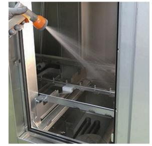
Unscrew the end caps from the wash arms (and prewash arms, if so equipped). Thoroughly spray down the inside and outside of the arms using a spray hose.
