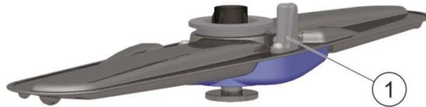
5. To ensure that the sensor detects the rotation of the washing arm, remove all dirt particles and ferrous particles sticking to the magnet (1).
