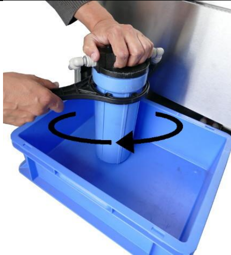
1. Use key to unscrew casing by turning clockwise. Position base drip tray!
