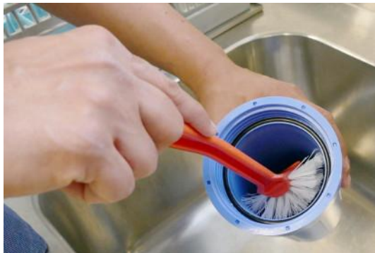
3. Thoroughly clean and rinse the filter housing. Remove deposits.
