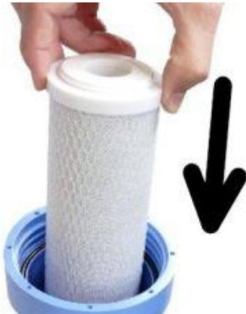
5. Insert the new filter cartridge, which has already been thoroughly rinsed, both inside and out. Check if the seals sit correctly.
