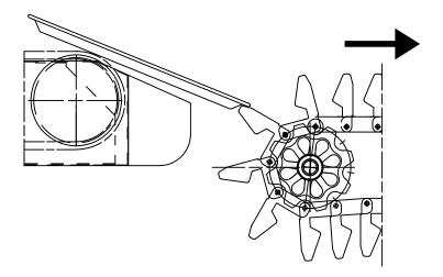
If the tray runs against the tray transport finger during infeed (see illustration below), the disk **must** be turned slightly **opposite to the transport direction**.
