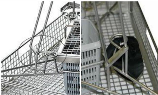
Lift safety device, place inner mask on bracket and secure.
