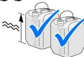
3. Check the canister fill level.
