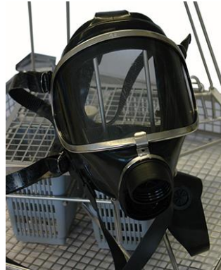
Hang the mask on the upper sealing edge on a bracket.
