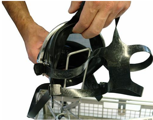
Lift safety device, place inner mask on bracket and secure.
