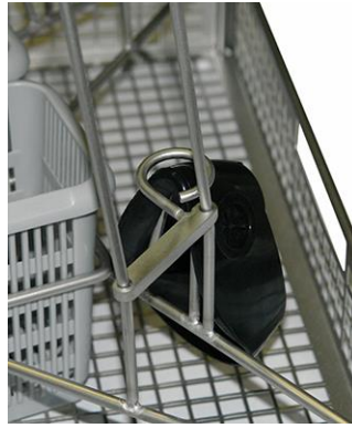
Lift safety device, place inner mask on bracket and secure.
