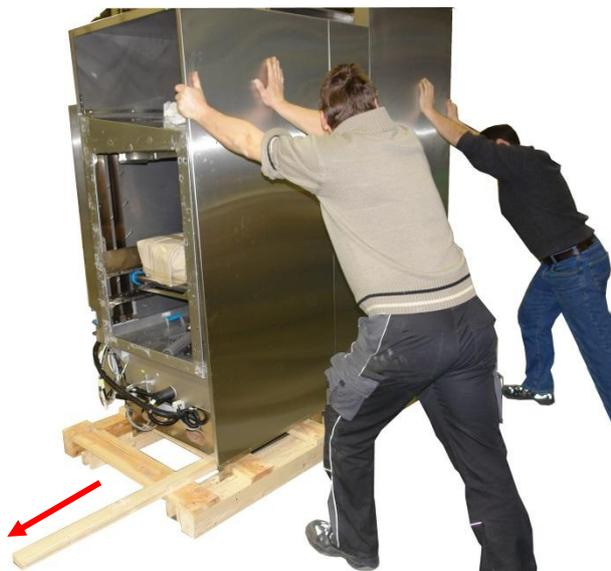
All the glands of the transport packaging are unbound, the machine will be lifted on one side and all the great longitudinal beams can now be pulled out without any effort under the machine.
