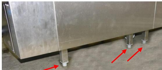
An open-ended 27 mm spanner is needed to adjust the cleats of the appliance!
