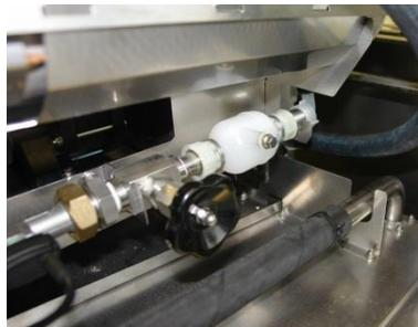
The connection for the rinse agent supplier is provided in this mixing chamber.
