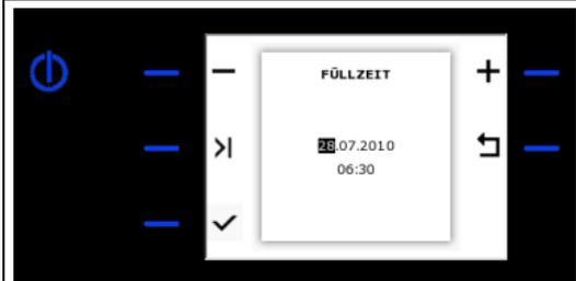
Enter the required date and time. Press the +/- button to change the value in the selected field. Then press >| to move to the next field.
