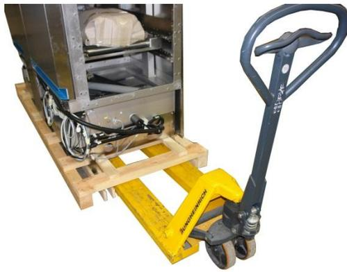
Incoming goods should only arrive on these wooden frames. The packing is specifically designed to allow the appliances to be moved safely and securely using a pallet truck.
