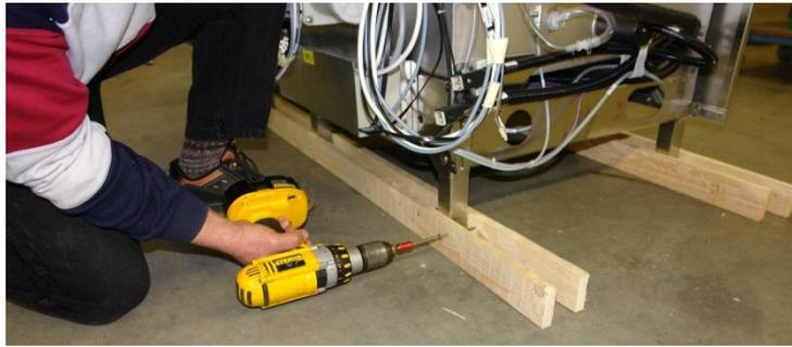
All the screws and bolts of the packing are now removed.
