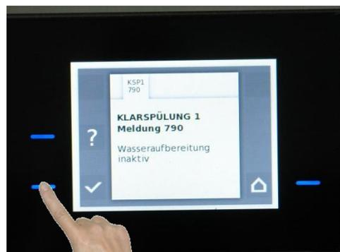
If an acknowledgment option is not available in the form of a checkmark on the display, it means that no water is available on-site or that the on-site water supply is blocked by a closed stop cock. When the on-site water supply is available again, the water treatment plant can be reactivated (see image to the left). If this is not the case, please inform the appropriate service representative.
