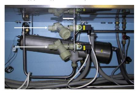
In order to avoid damage during transportation, water pipes may in certain circumstances be dismantled. These must be re-installed before commissioning.
