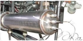
Temperature safety limit switch on the drying heating register:
