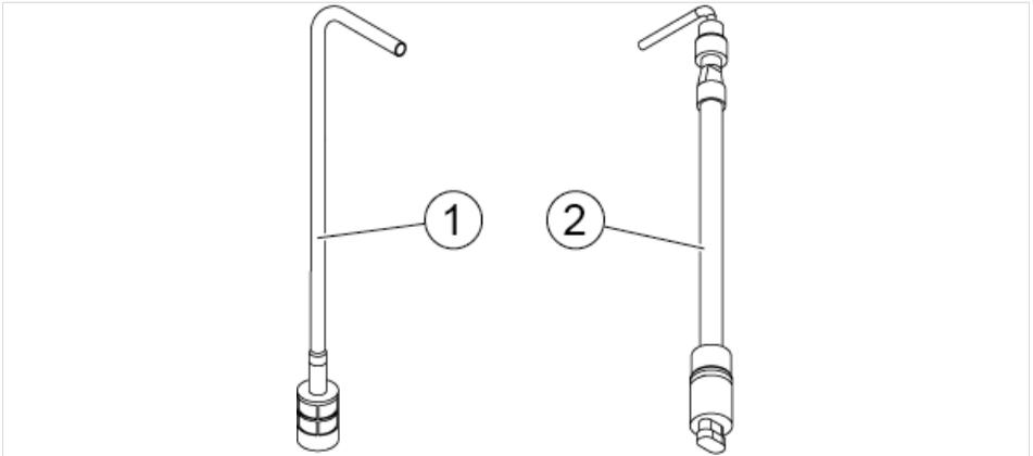
1. Insert the rinse aid suction lance (1) and the detergent suction lance (2) in the corresponding canister.
