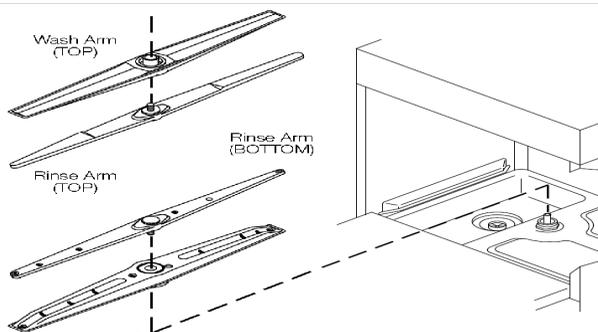
5. Insert the filter, the tank cover sieve and the wash systems.
