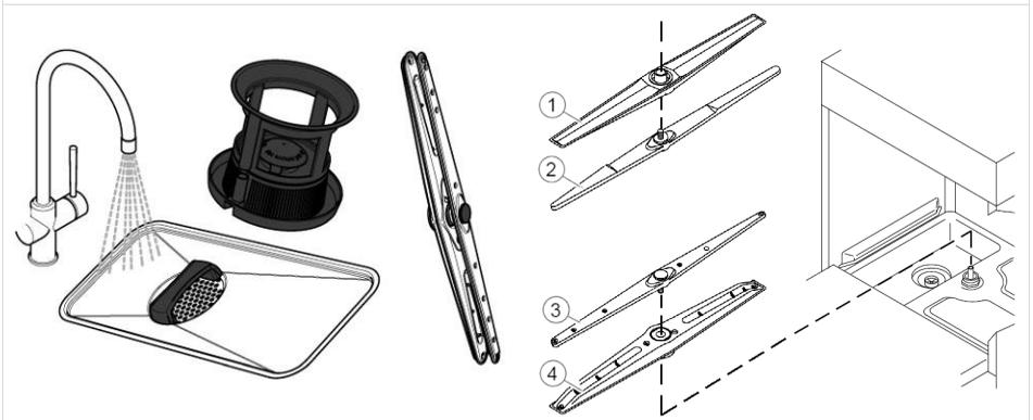
5. Rinse the filters, sieves and the wash and rinse arms thoroughly under running water. When doing this, pay particular attention to the nozzles.
