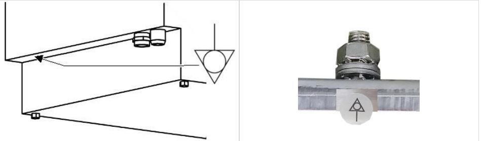
The screw for equipotential bonding is located on the back of the machine near the media connections.
