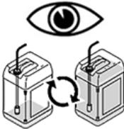
1. Remove the suction lance from the empty canister and insert it into a full canister.
