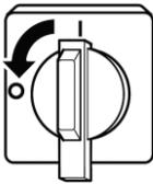
1. To do this, turn the local main switch to OFF and ensure that it cannot be switched back on again.
