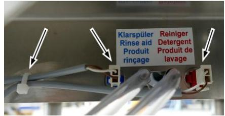
4. Secure the cables of the two suction lances to the clip provided with a cable tie. Depending on the machine type, the cables can be routed to the left or right.
