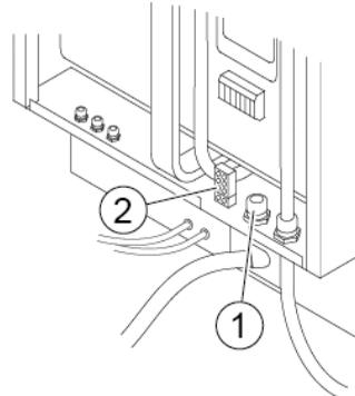
2. Route the electrical supply line through the strain relief (1) from below and to the main connection terminal block (2).
