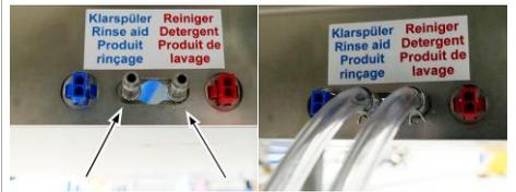
1. Attach the labels for rinse aid (blue) and detergent (red) to the hose and cable of the suction lances using cable ties. The suction lances are identical in construction. The labels are used to distinguish the canisters.
