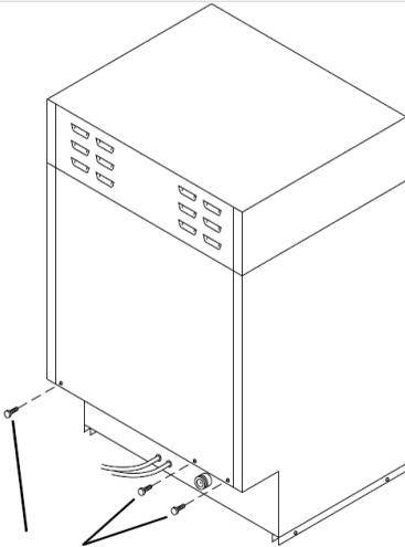
1. Remove and retain the three screws on the bottom of the rear panel.
