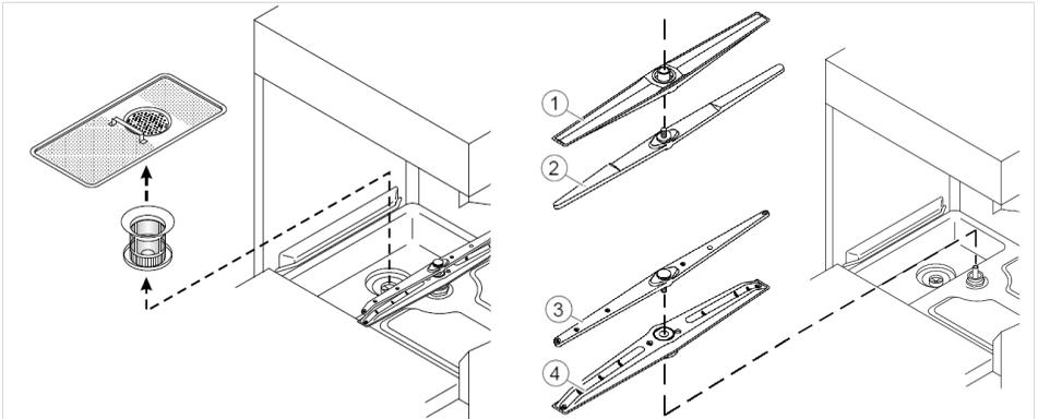
3. Remove the tank cover sieve and the filter. All parts to be cleaned are blue or have a blue handle.
