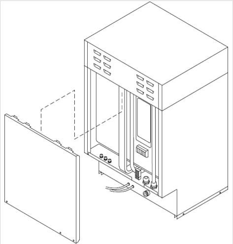
2. Carefully slide the rear panel down to free the retaining clips along the casing.
