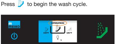
During the wash cycle,  $\bigcirc$  is lit in green, and the display will read **OPERATION**. A blue progress bar moves across the display to show the remaining time in the cycle.
