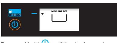
Press and hold U until the display reads FILLING.
