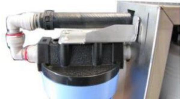
4. Secure the fresh water supply line to the pre-filter with a spring band clamp and connect the bend plug connection.
