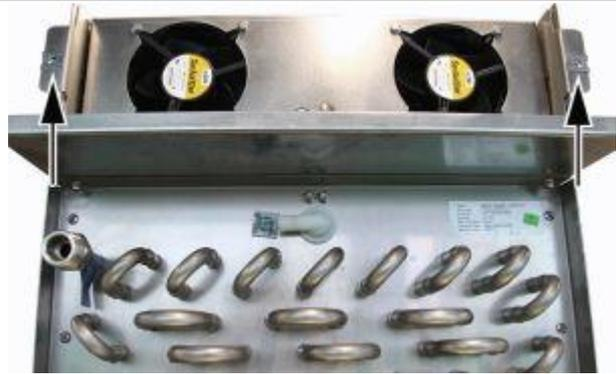
6. Slide the four clips onto the holes on the sides of the fan unit.
