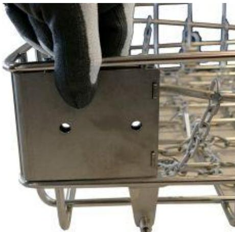
5. Fit the mounting plate for the outside of the rack.
