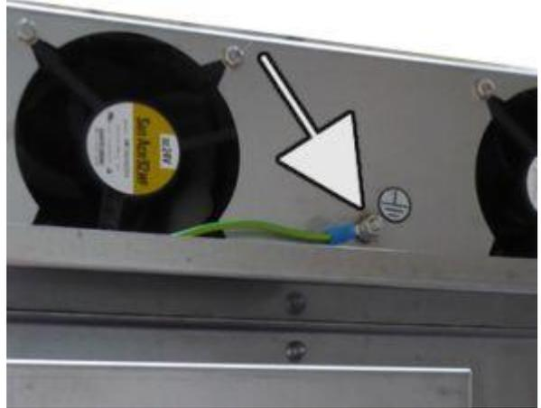
13. Attach the protective conductor on the side with connection plan Z.
