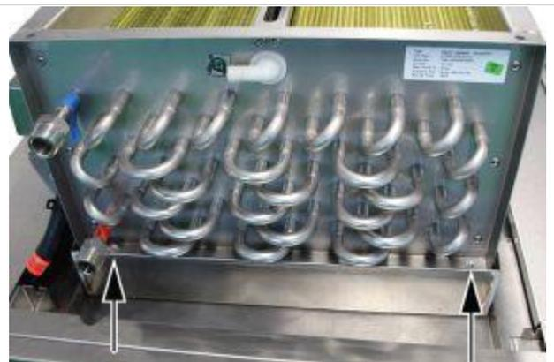
2. Secure the heat exchanger unit with 4 M5 safety nuts.
