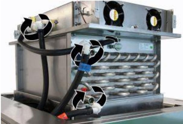
11. Connect the hoses and tighten them by hand. Secure the upper hose on the front with a spring band clamp.
