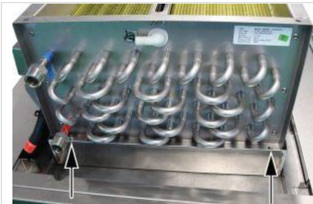
1. Place the heat exchanger unit on the dishwashing machine and insert the threaded bolts on the dishwashing machine through the holes in the heat exchanger unit. Position the connections for the hoses on the left-hand side.
