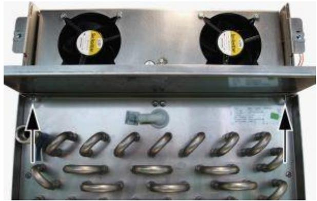
4. Place the fan unit on the heat exchanger unit and guide the threaded bolts of the fan unit through the holes in the heat exchanger unit.
