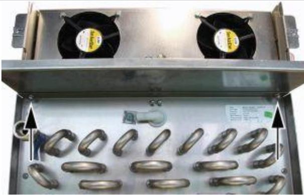
5. Secure the fan unit with 4 M5 safety nuts.
