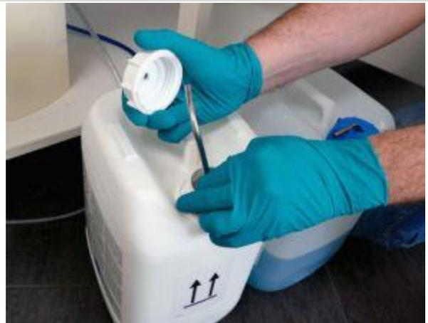
3. Guide the suction lances into the canisters and through the hole in the canister cover. Screw on the canister covers tightly.
