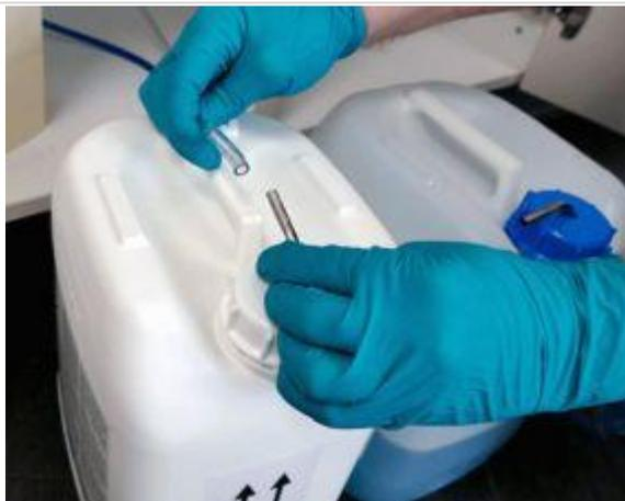
4. Connect the transparent hose to the suction lance in the white canister for detergent. To secure in place, squeeze the clamp at the connection and release it at the correct position.
