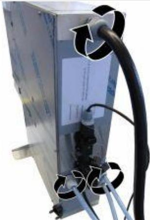
11. Tighten the hoses from the outside and attach the cover.
