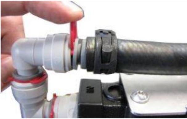
5. Fit the circlips.
