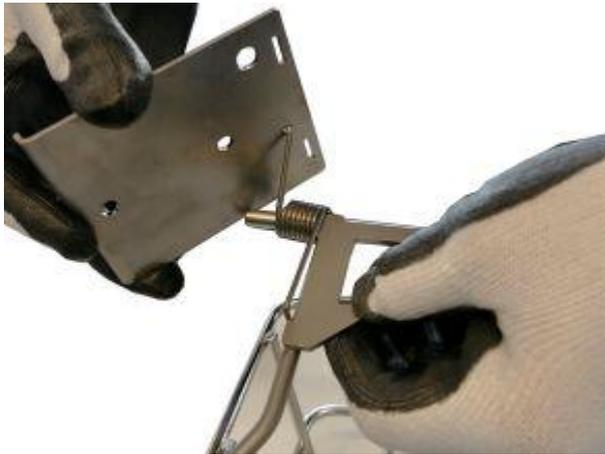
1. Place the spring on the axle of the hold-down grid as shown and hook the right-hand leg of the spring onto the hold-down grid from below.
