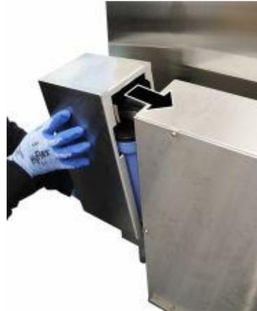
19. Hook in the pre-filter casing and push it down.
