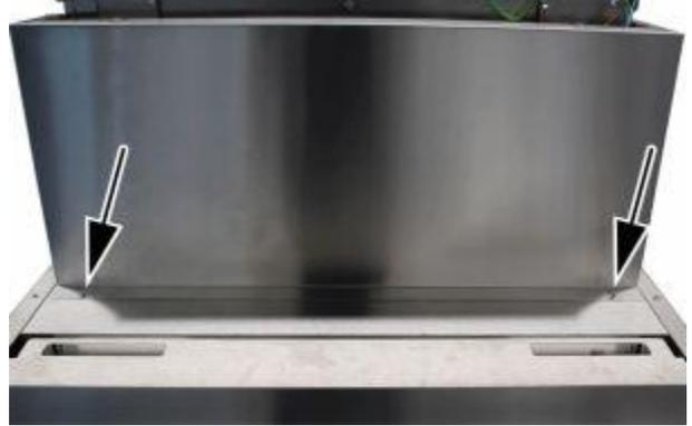
14. Slide in the heat exchanger unit casing from the front and hook it onto the sides.
