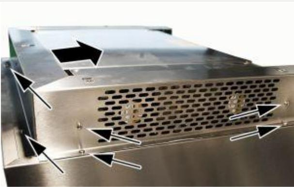
17. Push in the fan unit casing from the front. Secure the casing with 4 self-tapping screws per side and 2 self-tapping screws on the front.
