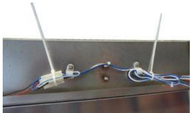
12. Lay the cables on the machine according to the cable length and secure them with the enclosed clamps.
