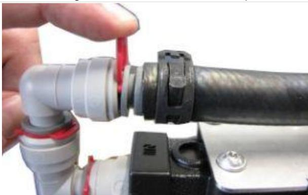
5. Insert the circlips
