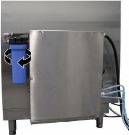
18. Insert the filter element and screw in the pre-filter hand-tight.
