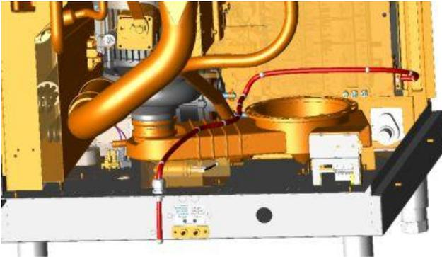
1. Insert the cable at the rear of the machine at the cut-outs provided. Lay between the wash pump and tank in the direction of the electrical box as shown and fix in place. It is permitted to lay the cables with the existing load circuit (230 V/400 V).
