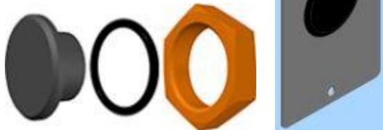
12. If the solid dosage is not used, the hole for the dosing connection in the wash chamber must be closed with the sealing plug, the O-ring and the hexagon nut. The grommet of the cover plate must be replaced with the sealing plug.
