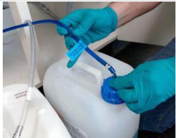
5. Connect the blue hose to the suction lance in the blue rinse aid canister. Tighten the clamp on the connection.
