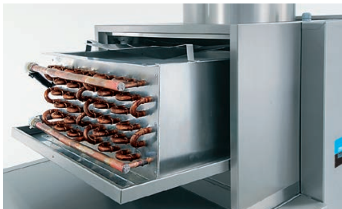
MEIKO heat recovery: Large 60 m 2 surface of the heat exchanger. For cleaning, the cooling register can be pulled onto the top of the machine. At the same time, the front plate serves as a trough.
