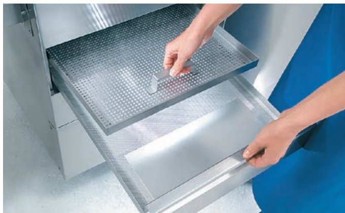
Double sieve system in the optional pre-wash area: Filters the smallest food particles out of the water and thus keeps them away from the machine's alkali wash zone. This reduces the amount of dirt in the wash water, reduces the regeneration water quantity and enables savings on detergent.
