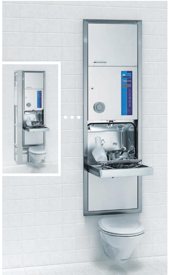
Cleaning and disinfection appliance *TopLine 30* with WC outlet for the bathroom in the patients' room, e. g. on the isolation ward. With mounting frame and complete piping as well as central connections for all commercially available WC types.
